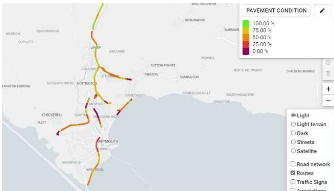
Illustration of cycleway condition (0% - purple being poorest condition)
